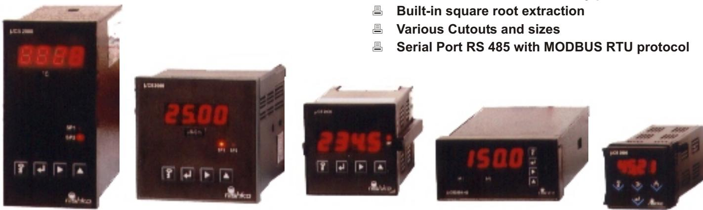
The CS 2000 series Digital Process Indicators are precision instruments used for display of Linear / Non linear process parameters. The same unit can be configured at site to accept inputs from two-wire, three-wire or four-wire transmitters or temperature sensors. The thermocouples and RTD's are linearised. Two programmable set-points and isolated retransmission output is also provided.
